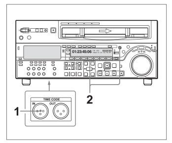
**1** Connect the time code output of the external time code generator to the TIME CODE IN connector.
